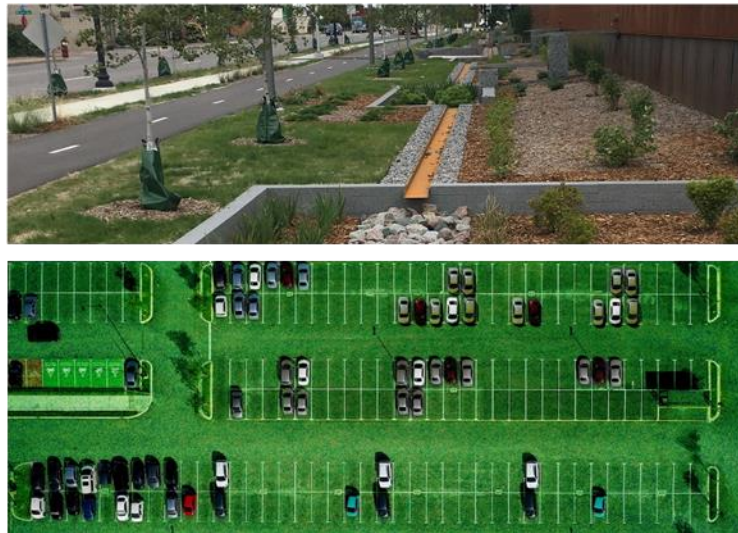
Figure 28. Establishing green (grass) corridors around open parking areas that will facilitate the infiltration of surface waters into the ground.
